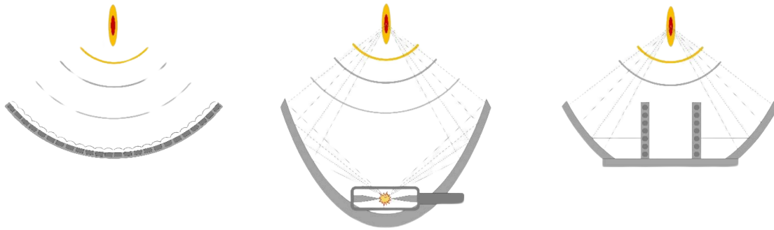
Fig. 2: Schematic illustrations of (left) piezoelectric, (centre) electrohydraulic, (right) electromagnetic shock wave generation principle. ©RWTH Aachen University, Germany
